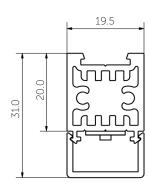
The Sideways Sally 20R extrusion is a compact uplight/downlight solution providing powerful LED lighting. A versatile system suitable for various mounting options, Sideways Sally 20R can be surface mounted, wall mounted and suspended. The concealed mounting clip provides a quick and secure fixing to joinery. Both wire and rod suspension options are available for the Sideways Sally 20R extrusion.
