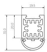
The Sideways Sally 20C extrusion is a compact uplight/downlight solution providing powerful LED lighting. A versatile system suitable for various mounting options, Sideways Sally 20C can be surface mounted, wall mounted and suspended. The concealed mounting clip provides a quick and secure fixing to joinery. Both wire and rod suspension options are available for the Sideways Sally 20C extrusion.
