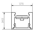
Much like its close cousin, Downhill Dan 14, Flat Freddie 14 is a compact solution providing "dot-free" lighting. A versatile system suitable for various mounting options, Flat Freddie 14 can be surface mounted, recessed or suspended. Both wire and rod suspension options are available and a simple method of recessing into plasterboard ceilings provides a clean, trimless look.
