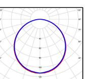
C0 - C180 - C90 - C270 Polar curve for 1340 lumen LED strip with opal diffuser.
