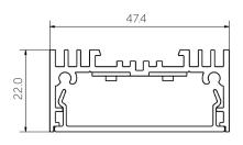
The Downhill Dan 22 extrusion is our most powerful downlighting system. Utilizing two LED strips mounted side-by-side, this profile is ideal for applications where maximum light output is key. A versatile system suitable for various mounting options, Downhill Dan 22 can be surface mounted, recessed and suspended. Both wire and rod suspension options are available for the Downhill Dan 22 extrusion and the recessing systems for plasterboard ceilings and walls create a beautiful trimless finish.
